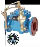
Apollo control valves are ideal for a wide range of commercial and industrial applications, wherever the flow, pressure or level of liquids needs to be controlled. Hydraulically operated diaphragm main valve automatically controls non-corrosive, non-abrasive fluids by means of a wide range of pilots.
