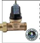
Economy, compact and corrosion-resistant. Supply pressures up to 400 psig; built in by-pass relieves excessive pressure buildup. Working temperatures to 180°F, 50 psig standard factory setting; easy screw adjustment. Meets ASSE, CSA and ANSI standards and is listed with IAPMO. FNPT, sweat union, PEX, PUSH, ApolloXpress or FNPT union connections available. Sizes: 1/2" to 1".
